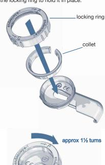
The locking mechanism aligns the endoscope with the rear camera lens for endoscopic imaging and prevents the endoscope from accidentally detaching - even if not fully tightened.
