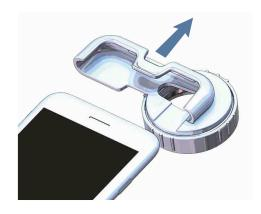
**REMOVAL:** loosen the locking ring by turning it anticlockwise until the endoscope is released.
