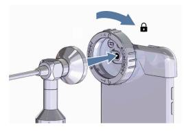
Secure the endoscope by turning the locking ring clockwise and tightening it by hand.
