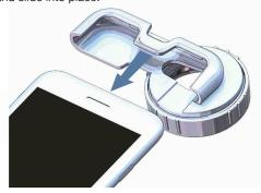
Secure to the phone by firmly pressing the catch over the top hand edge on the adapter till it latches over the speaker port with a snap.
